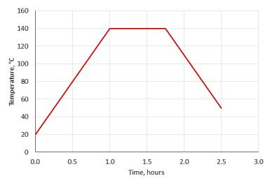
Alternative cure cycle to optimise surface finish for cures at 140°C:
