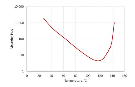
Plate-on-plate, ambient temperature 25°C, shear rate 20s<sup>-1</sup>, ramp rate 2°C/min:
