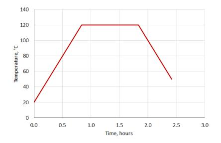
Alternative cure cycle to optimise surface finish for vacuum bag/oven cures at 120°C:
